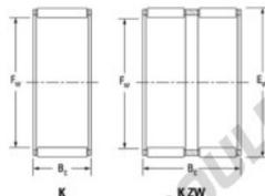
Radial needle roller and cage assemblies
