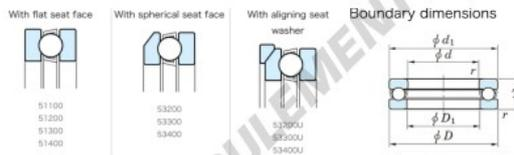
Thrust Ball Bearings - Single Direction
