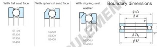
Thrust Ball Bearings - Single Direction
