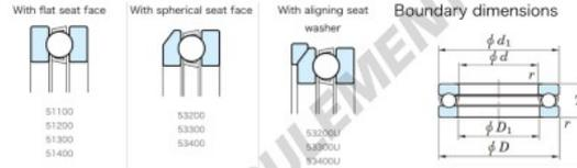
Thrust Ball Bearings - Single Direction
