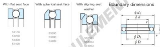
Thrust Ball Bearings - Single Direction
